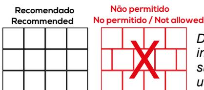
Do not allowed laying in an overlaid position such as "bricks". Please use continuous joints.
